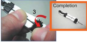
Set the fiber along the groove tightly before closing the back cover
