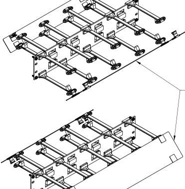
FRONT AND REAR PANEL SWINGS DOWN OR UP FOR CABLE ACCESS
