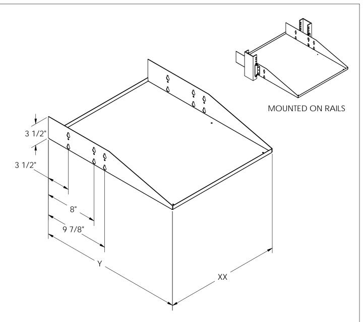
STATIC CAPACITY 150LBS MOUNTING BRACKETS INCLUDED
