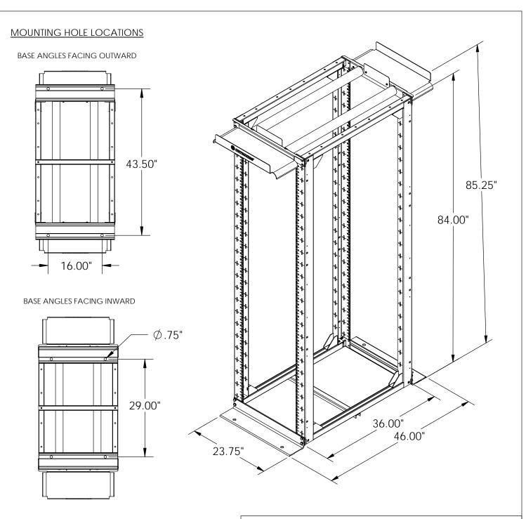
TESTED TO UL2416 WITH A WEIGHT LOAD OF 2000LBS.
