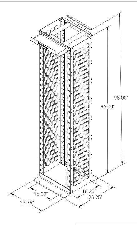
TESTED TO UL2416 WITH A WEIGHT LOAD OF 2000LBS.
