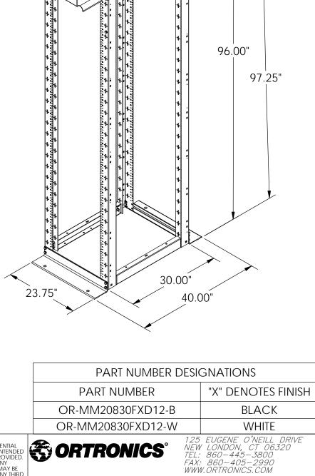
TESTED TO UL2416 WITH A WEIGHT LOAD OF 2000 LBS.
