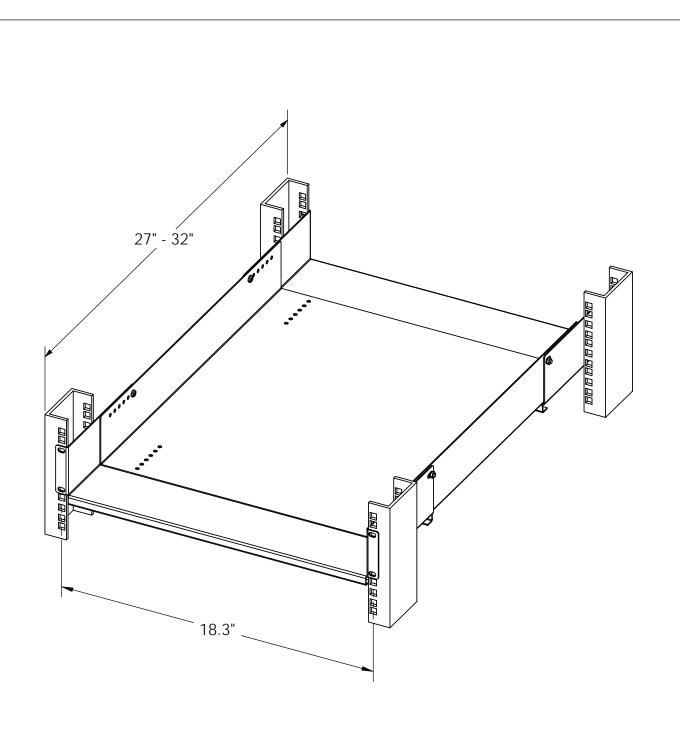
**CENTER LOAD RATING 125 LBS** DISTRIBUTED LOAD RATING 300 LBS MOUNTING HARDWARE INCLUDED
