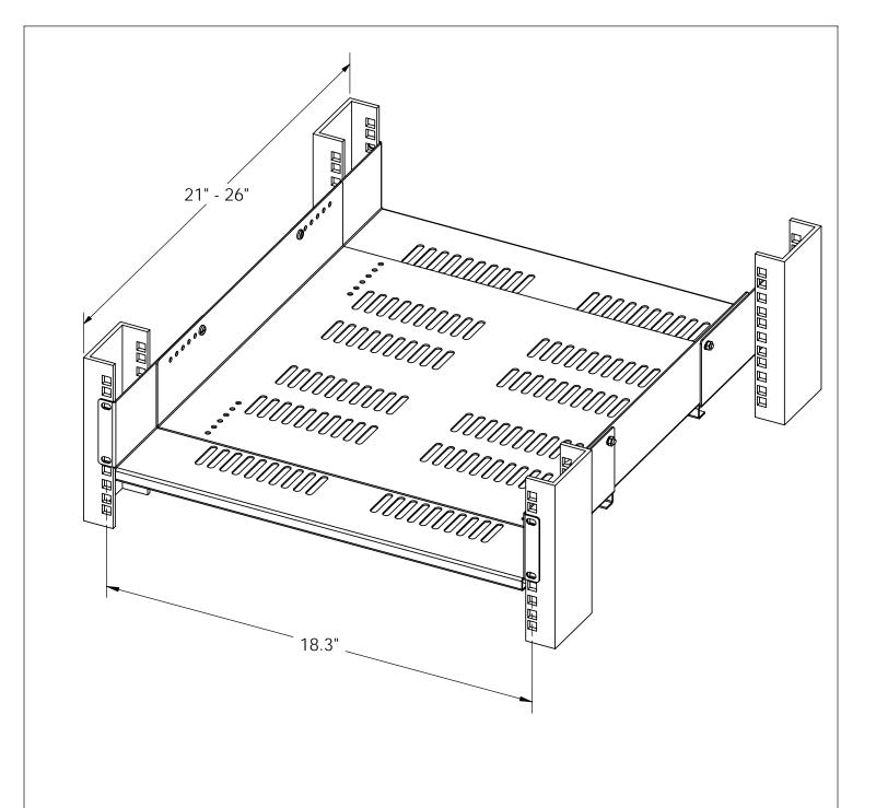
**CENTER LOAD RATING 125 LBS** DISTRIBUTED LOAD RATING 300 LBS MOUNTING HARDWARE INCLUDED
