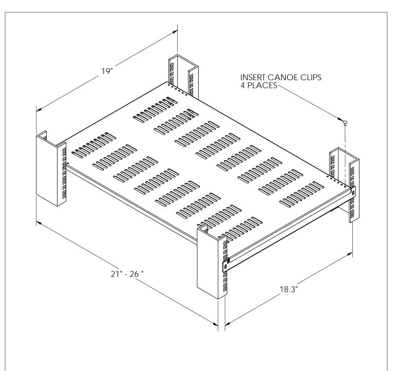
**CENTER LOAD RATING 125 LBS** DISTRIBUTED LOAD RATING 300LBS MOUNTING HARDWARE INCLUDED
