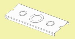
The DataCab wall mount cabinet comes standard with four removable cable knockout panels on the rear section. Each section contains one knock-out that can be 1-3/8" or 2" diameter and two knockouts that can be 7/8" or 1-1/8" diameter.
