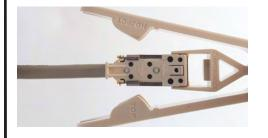
STEP 1: HOLD THE TERMINATION TOOL IN ONE HAND AND THE JACK AND CABLE IN THE OTHER. ALIGN "TOP" MARKING OF JACK WITH "TOP" MARKING OF THE TOOL.
