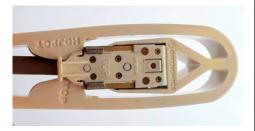
STEP 3: SQUEEZE THE TOOL TOGETHER UNTIL BOTH SIDE LATCHES ARE ENGAGED AND CLICK. GENTLY PULL CABLE TO ENSURE PROPER TERMINATION.
