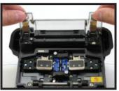
Internal Heat Oven on Splicer
