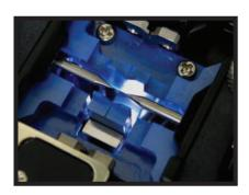
3. It is recommended to replace electrodes after 1000 arc discharges.
