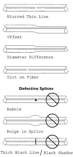
White lines or faint lines in splices should not be considered automatic failures. Without testing through the splice there is no accurate way to evaluate the splice. Black lines or bubbles in the splice should be replaced.
