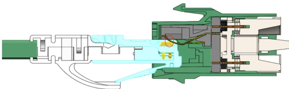
The concern about contact plating damage from arcing can be **successfully addressed by segregating any potential arcing to a location separate from the fully mated contact area of both the plug and jack.** This approach to the spark gap mitigation has been confirmed and has also been referenced in other position papers on this topic.
