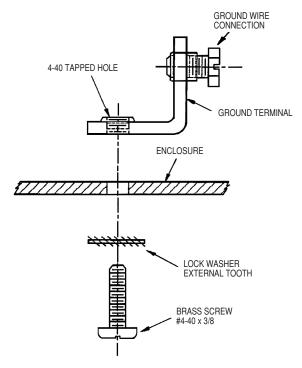
Assemble ground terminal as shown above.
