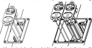
B. Mount the device in box by sandwiching the device to the box with the intermediate sub-plate using provided #6-32 x 3/4" pan head mounting screws. Note: Orient the Sub-plate to say "THIS SIDE UP". For the two port, attach the device to the box by screwing the strap directly to the box using provided #6-32 x 3/4" pan head mounting screws.
