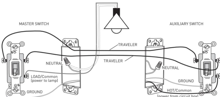
Fig. 2: Typical 3-Way Switch Wiring
