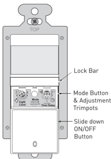
**Fig. 6: Sensor Adjustment Controls**
