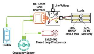
a value established by auto or manual calibration.) If the light level falls below the On Setpoint for more than 20 seconds (On Time Delay), the photosensor will restore a higher level.
