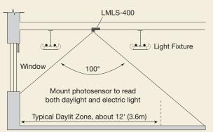
Sensor placement is the first step to ensuring proper opration. The rule of thumb for the LMLS-400 is to place the sensor two window heights deep into the space, in a location that will not be affected by uplight contributions from nearby fixtures.
