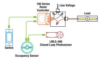
Turning the lights ON after the photosensor has turned them OFF in response to daylight (permitted by Allow Override setting of "Yes") overrides photosensor control for 2 hours (selected Override Time), or until the lights are turned OFF. Turning the lights OFF (via the switch or the occupancy sensor) disables photosensor control because the Hold Off setting is "No."
