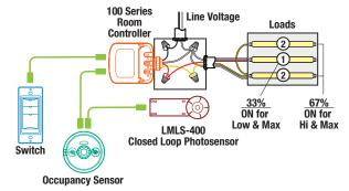
a value established by auto or manual calibration.) If the light level falls below the On Setpoint for more than 20 seconds (On Time Delay), the photosensor will restore a higher level.
