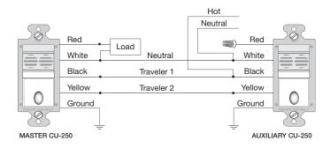
Up to four multi-location sensors may be connected together. For details on connecting RH-253s for multi-location control, see the RH-253 cut sheet.
