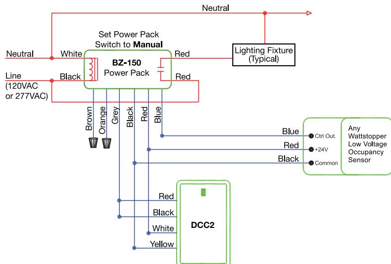
As shown, the LED on the DCC2 is always on, serving as a locator. To disable, disconnect and cap the yellow wire.
