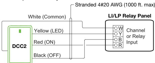
As shown above, the DCC2 LED is a Pilot Light. To use the LED as a locator, connect the yellow wire to the panel's 24V supply.
