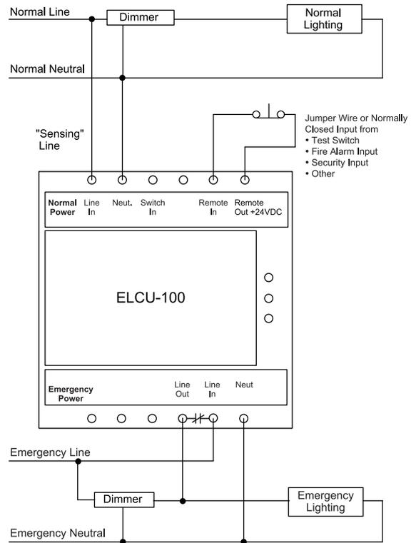
When wired as a shunt, the switching line is not used.
