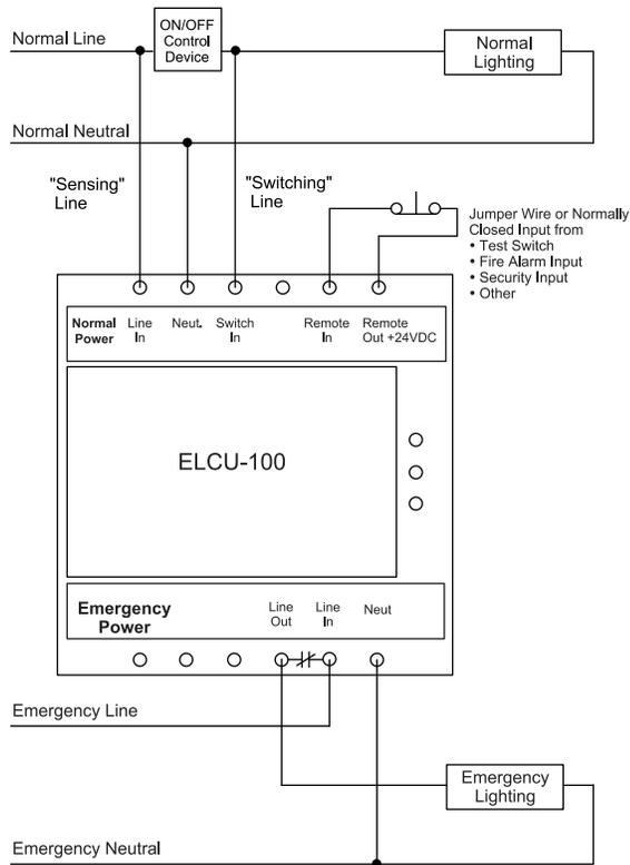
When wired as a control device, the ELCU-100 receives a switching signal from the output of the control device (relay, switch, power pack, etc.)
