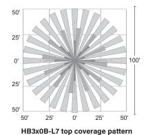
For high bay applications, the HBL7 is designed for mounting at heights between 20' to 40', with a coverage area up to 100' in diameter when mounted at 40'.
