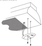
HB340 has no back box, for surface mounting to bottom of fixture. Back box can also be removed from other
