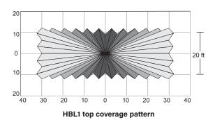
The HBL1 is designed to detect walking motion when mounted at 40' above the floor. When mounted at 40', in optimal conditions, the lens has a 60' linear detection range.
