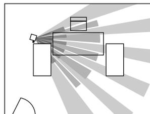
The IT-200 monitors an area of up to 150 ft<sup>2</sup> (13.9m<sup>2</sup>). The unit should be placed near the light source with the light pipe aimed at the light and the lens facing the occupant's main work area.
