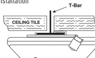
The IT-200 simply clips to a T-bar of a ceiling tile — no wiring is needed. For installation onto other surfaces, the unit comes with a flat bracket and double-stick tape.
