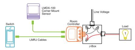
Plug DLM local network components together in any configuration using Cat 5e cables with RJ45 connectors.
