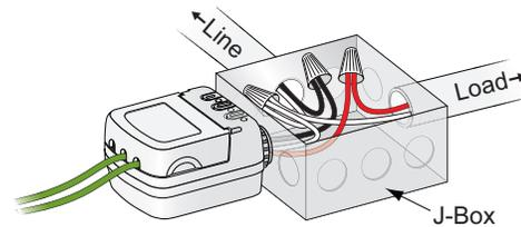
Mounting outside a j-box (plenum space). Two LMPL-101 and/or LMRC-100 Series Room Controllers may be mounted to the j-box.
