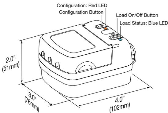
LMPL-101 Plug Load Controllers include a 1/2" (12.7mm) threaded nipple and locking ring.
