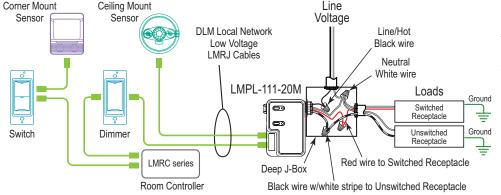
Plug DLM local network together in any configuration using Cat 5e cables with RJ45 connectors.
