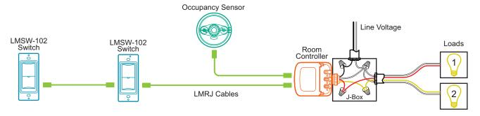
Plug DLM local network components together in any configuration using Cat 5e cables with RJ45 connectors.
