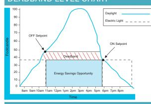
If the LS-102's photosensor lighting level drops below the on setpoint, the lights will remain on. If the sensor's lighting level rises above the off setpoint, the LS-102 will automatically turn the lights off. If the sensor's lighting level remains in the predetermined deadband range (25%, 50%, 75% or 100%) the lighting will be passive until the sensor's level reaches the high or low setpoints.
