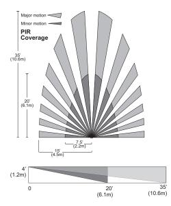
For best performance in single location applications, Wattstopper recommends using this sensor in spaces no larger than 15' x 12'. In multi-way applications, each connected sensor expands the coverage area.
