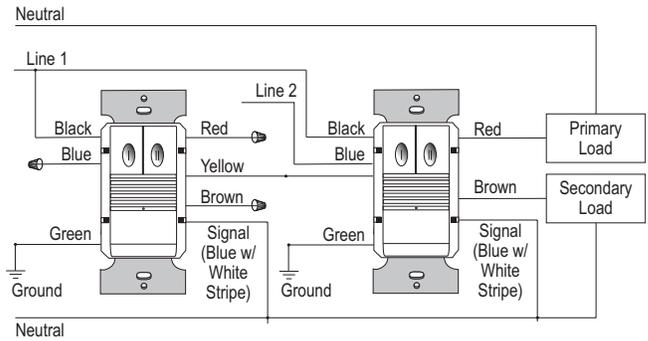
Signal wire connects to neutral. Signal wire can connect to ground in replacement or retrofit application
