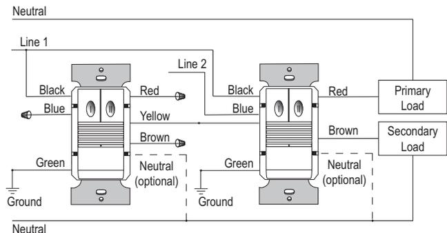
Simple optional neutral connection allows installation in any 2-wire or 3-wire application. When used in a multi-way application, all devices in that space must be wired using the same method of either with neutral or without neutral.
