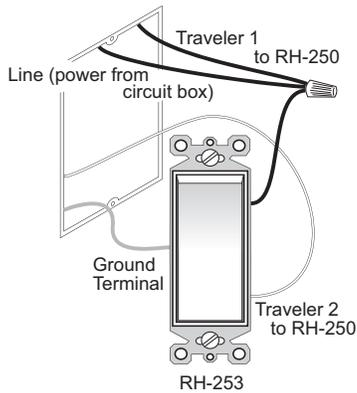
The RH-253 may be used with the RH-250, as shown in these drawings, or with a CH-250, CD-250, CU-250 or RD-250 multi-way sensor in place of the RH-250.
