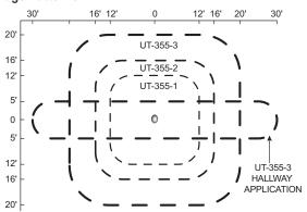
Coverages shown represent half-step walking motion when sensor is mounted 8'-10' high. Actual coverage can vary for each application depending on the shape and use of space and the obstacles present.
