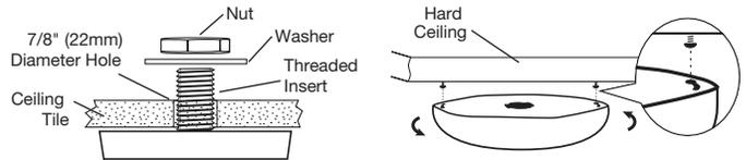
The WRC-TX is designed to mount either in an acoustic tile or on a hard surface
