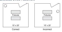
For enclosed spaces, place sensors as in Figure A. Sensors placed as in Figure B may see out the door and cause false triggers.
