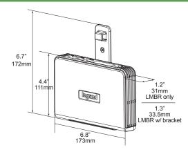
Wattstopper recommends mounting to a vertical surface, using the included T-shaped bracket, for optimum efficiency of wireless transmission/reception. 10' minimum and 100' maximum between LMBR-650 and LMRC-611MCC or LMBC-650.
