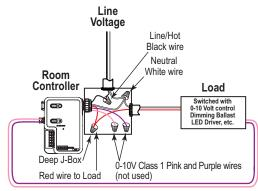
0-10V Class 2 Dimming control wires
