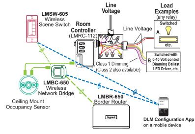
**Note:** For a single (non-networked) hybrid room, the LMBR-650 is not required. **Note:** the DLM Config App can only connect with the LMBC-650 to update firwmare or pair devices. You need an LMBR-650 and LMCS to commision a Hybrid room. For a single room, without an LMBR-650, LMCS can connect to the LMBC-65- via the LMCI.
