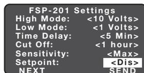
The Auto option invokes an automatic calibration procedure to establish an appropriate setpoint based upon the contribution of the electric light. As part of this procedure, the controlled load is turned on for two minutes to warm up the lamp, and then switched off and on eight times, terminating in an off state. After this process, a new setpoint value is automatically calculated.
