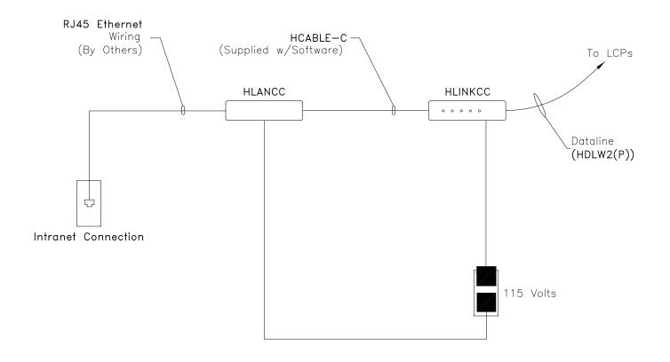
The TCP/IP Interface Module (HLANCC) connects to the Lighting Integrator (LI) Communication card global dataline through the HLINKCC Dataline Link using the HCABLE-C cable, and to the Ethernet side using a standard RJ45 connector. A 115V plug—in transformer is supplied to power the HLANCC. A PC running WinControl lighting control software connects to the LI dataline through the HLANCC via its own connection to the Ethernet network.
