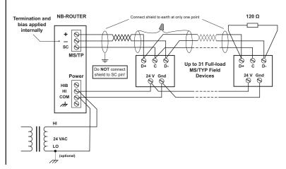
For MS/TP devices that use a power source separate from the NB-Router
