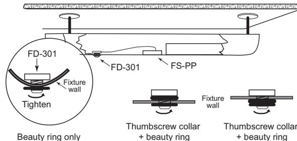
Figure 3: Installing in a light fixture
