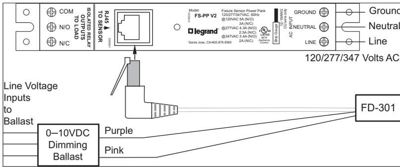
Figure 4: Basic wiring for daylight dimming control
