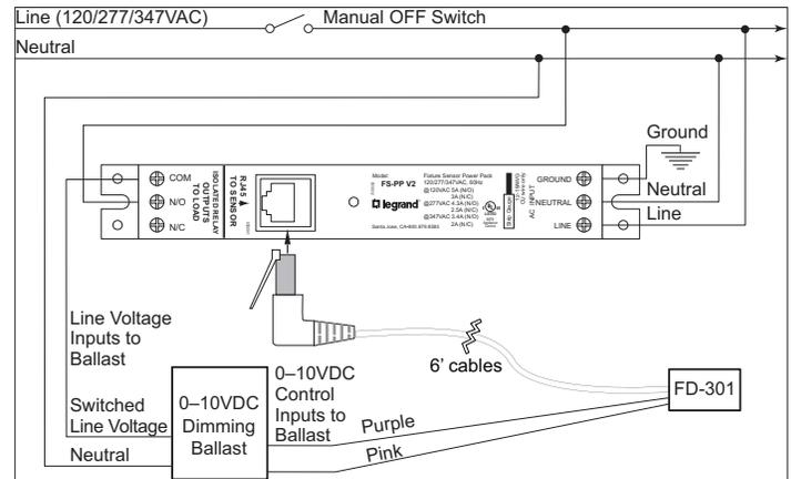
Figure 5: Wiring for daylight dimming w/ occupancy sensor ON/OFF control
