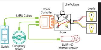
**CAUTION:** TO CONNECT A COMPUTER TO THE DLM LOCAL **NETWORK USE THE LMCI-100.** NEVER CONNECT THE DLM **LOCAL NETWORK TO AN ETHERNET** PORT - IT MAY DAMAGE COMPUTERS AND OTHER CONNECTED EQUIPMENT.
