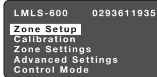
Zone Setup settings have been saved. The screen returns to the Daylighting Parameters menu.
