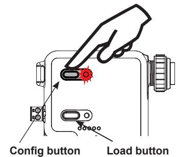
**NOTE:** Repeat steps 2 and 3 for each sensor and switch in the room, so that all devices are paired together in the same network. For each device, the load will toggle during step 3 and its config LED will turn solid green.
