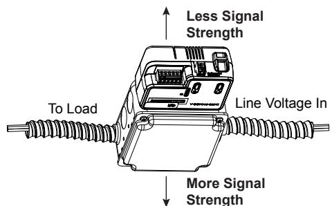
All line voltage wiring is #16 AWG. The relay is rated for up to 10A; total load for LMRC-611MCC not to exceed 10A. On/Off or 0-10V dimming loads can connect to any load relay.
