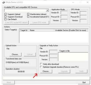
d. After choosing the correct file, press the "Upgrade" button to upload the file to the device. If a message pops up saying, "Your device was plugged in DFU mode" as shown below, click yes and continue.
