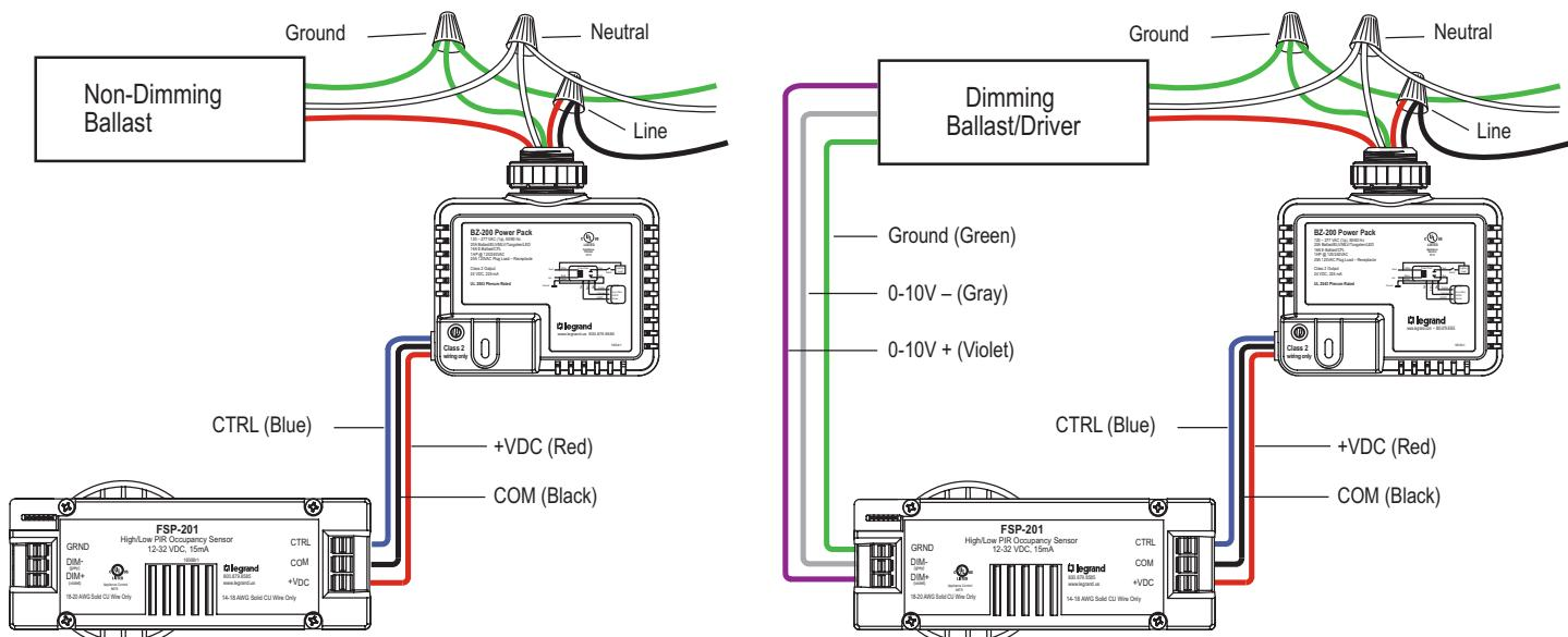
**NOTE:** The FSP-201 must be grounded to ensure signal integrity, not for safety ground.
