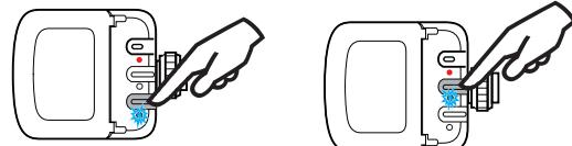
Blue LED ON when load is ON
