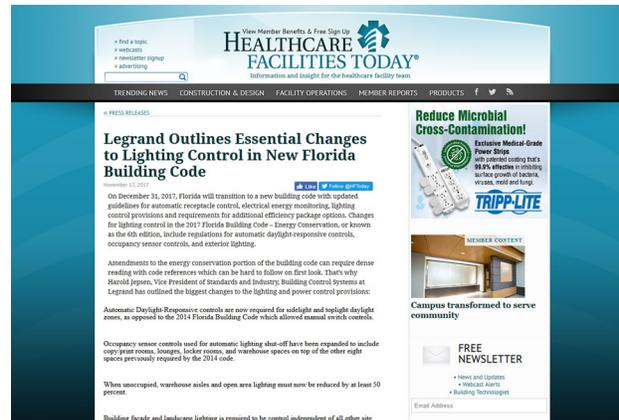
Automatic Daylight-Responsive controls are now required for sidelight and toplight daylight zones, as opposed to the 2014 Florida Building Code which allowed manual switch controls.
