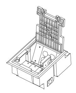
5. Low voltage cables may be brought out through a bushing in one of the device plates, or may be attached to a device that is mounted to the box or a device plate. The back or bottom covers do not need to be attached behind a compartment used for low voltage.
