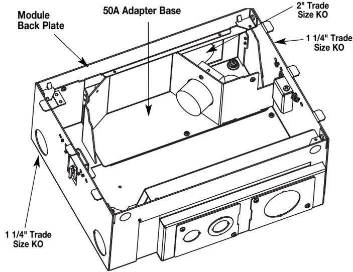
**Step 6.** Attach covers to the 50A adapter base and module back plate.
