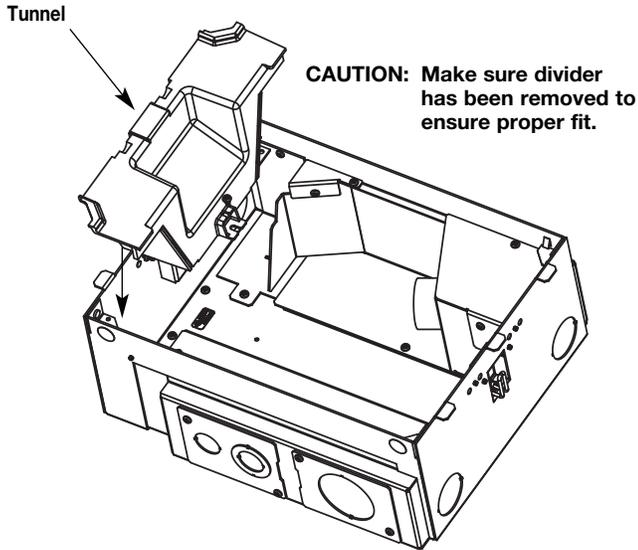
**NOTE:** To maintain the UL Listing, the tunnel must be installed when using the EFB-50A Adapter.
