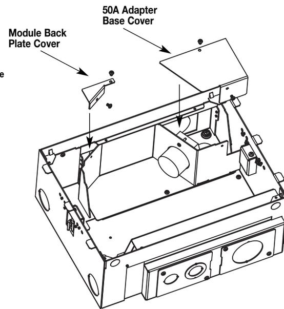
**Step 7.** Remove the tunnel divider on the side of the 50A adapter base. Cut off the divider shown at the score line with a hacksaw
