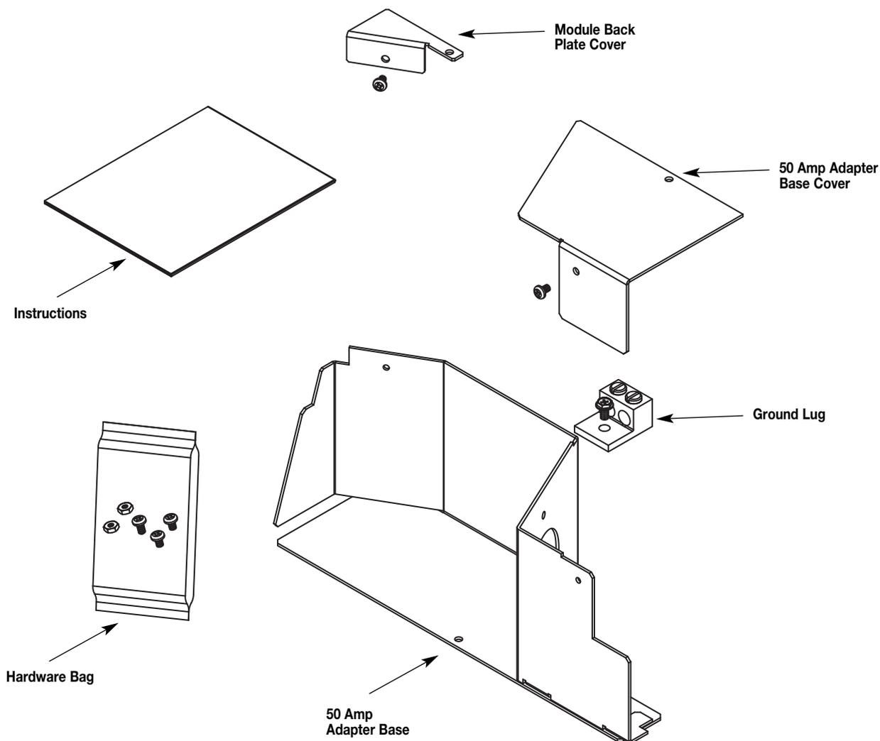
**Step 1.** The EFB-50A Adapter will only work with the plastic tunnel (EFB810-TUN). If you have the metal tunnel (EFB810S-TUN), you will need to order the plastic tunnel (EFB810-TUN).
