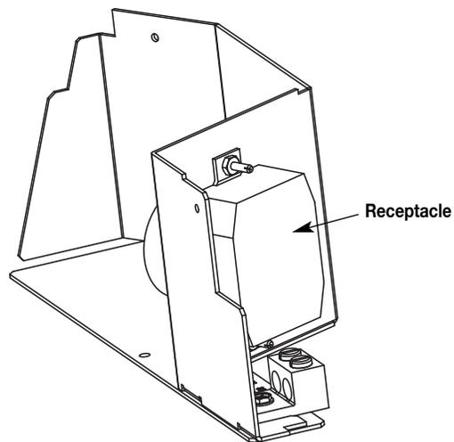
**NOTE:** Use two (2) hex nuts (included) to secure receptacle in place.
