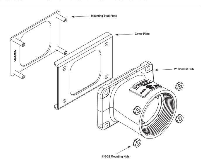
**Step 1.** Remove KO plate from desired location on the floor box for Hub placement. Use 1/4" hex head driver to remove the two screws as shown.
