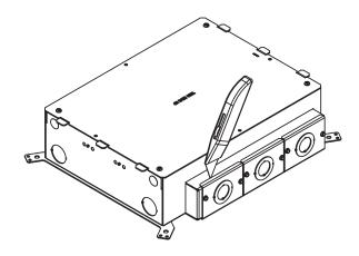
$\mbox{\bf Step 3.}\,$  Remove device plate on the inside of the floor box.
