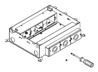
**Step 2. For On-Grade Boxes:** To facilitate the removal of the knock out plate, use a utility knife to score the paint around the edges of the plate as shown.
