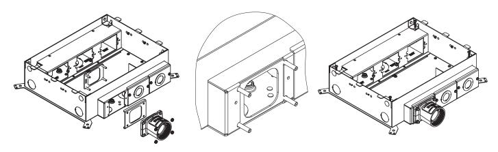
**Step 6.** Complete the installation by attaching 2 inch conduit to the Hub.
