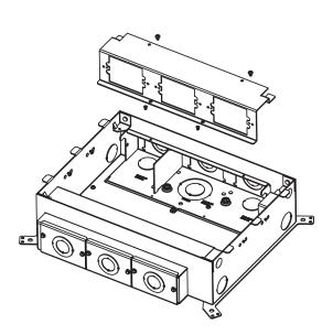
**Step 4.** Remove knock out plate by tapping the plate loose from the box as shown.
