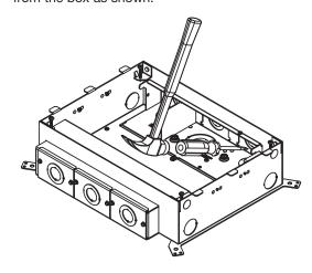
**Step 5.** Insert Mounting Stud plate on the inside of the floor box. Place Cover plate on the outside of the floor box. Position hub adapter onto the protruding studs and fasten together using the supplied #10-32 nuts.
